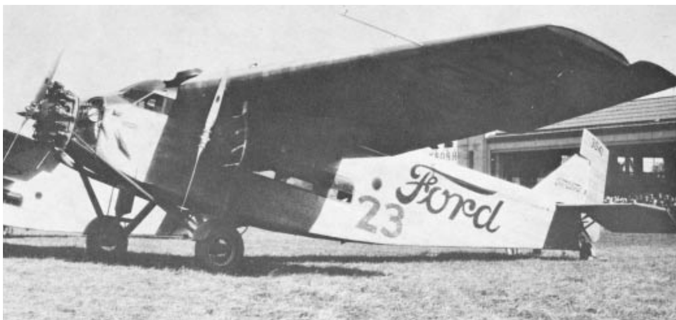
Ford #23, with unusual "Tri-Ford" designation on fin. The plane was listed as standard Whirlwind model in most tour publicity, however this picture indicates it had a Wasp in the nose position.
