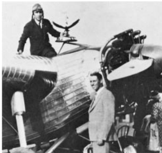
J. S. McDonnell, Jr., left, and Tom Hamilton with Metalplane at Spokane Air Races. The plane was designed to carry four passengers, who looked out, and down, through horizontal windows in bottom wing surface. (A. W. Walker)
