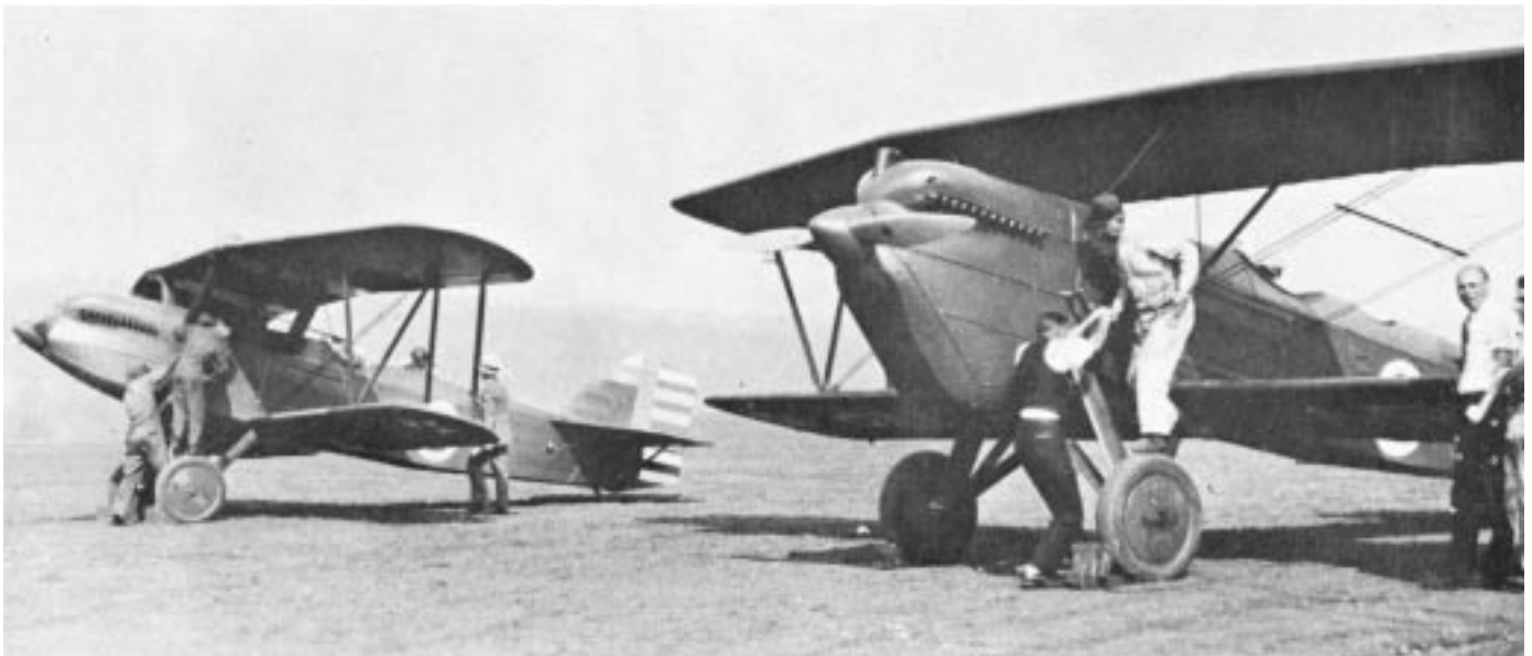
Typical scene: mechanics starting engines with hand-crank inertia starters. These are Curtiss Falcons at the Spokane Races, an O-1 at right, slicked up XO-13A, at left.
